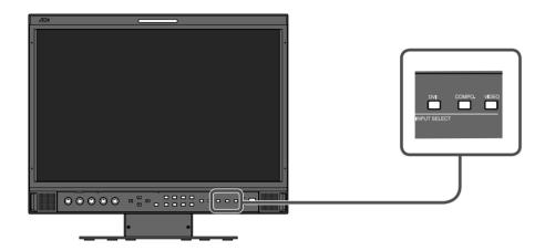
When the screen goes blank, and one or some of the INPUT SELECT lamps (DVI, COMPO., VIDEO) on the front control panel start flashing...
